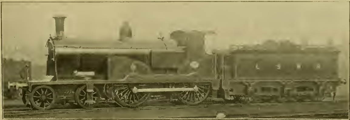
Locomotive with Water Tubes Across the Firebox. London & Southwestern Railway.
